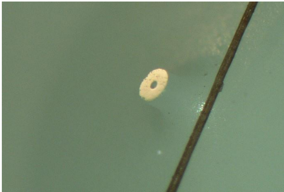
(image of a molded 50um hole in zirconia near human hair)
